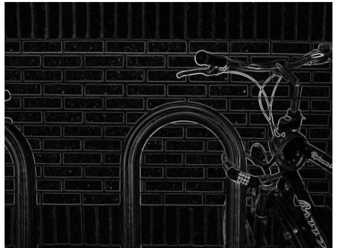
Gradient with Prewitt operator of grayscale image of a brick wall & a bike rack
