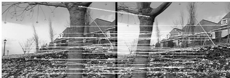
Fig. 3. Matches determined for a large baseline stereo pairs. Only 2–3 wrong matches are determined.
