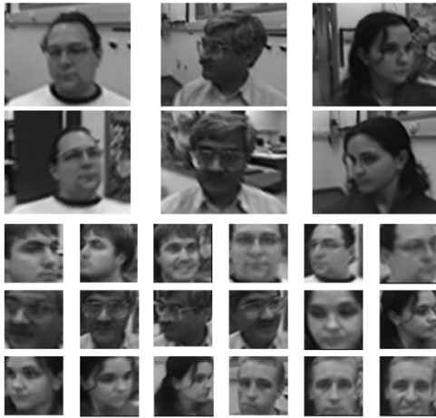
Fig. 15. Examples of the face images in the training and testing video streams. The left six are perspective views generated from the omnivideos, and the right face images are automatically extracted by the NOVA system. They show various face angles, sizes, expressions, backgrounds, and other perturbations that SFR needs to deal with.
