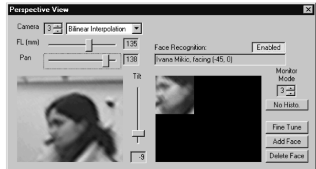
Fig. 9. Functional blocks of the NOVA intelligent room system. The lower window shows head tracking by ODVS perspective view generation and face recognition.
