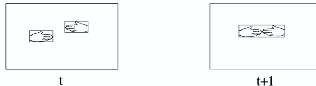
Fig. 2. A rectangle is formed around the hands or the big blob in occlusion
