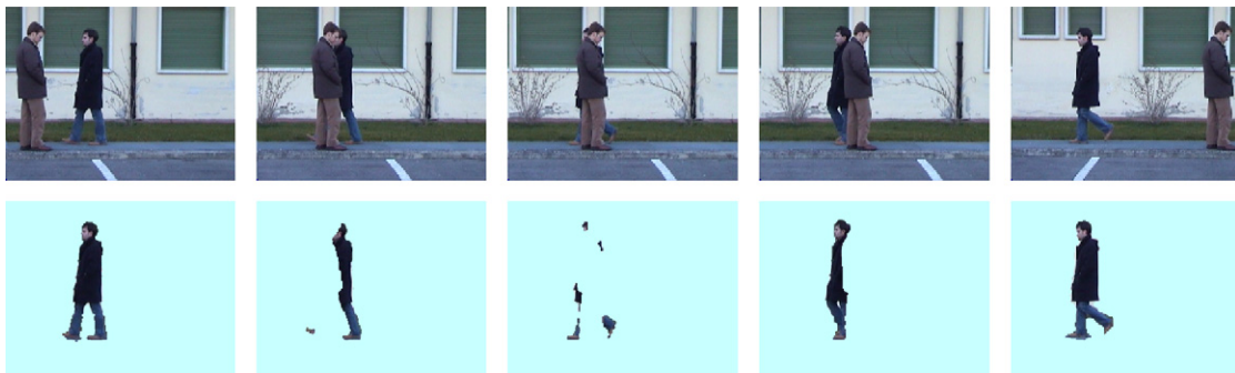
Fig. 11. Some selected frames from the “Pedone” sequence (top) and the result of the segmentation (bottom).
