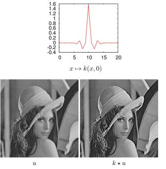
**Fig. 2.** Blind deconvolution of Lena image. Selecting the separable symmetric  $21 \times 21$  kernel k that maximizes the Sharpness Index of  $k \star u$  (u being the original Lena image, bottom left) results in a sharper image (bottom right) that reveal some details of the original image, while keeping noise and ringing at an acceptable level.
