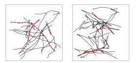
Fig. 13 Changing the acceleration variance. A sample of 20 trajectories generated using the PSMG algorithm, when the standard deviation of the acceleration magnitude ( $\sigma$ ) is 1 (left) and 4 (right). The points of two trajectories have been highlighted to show the speed. We study the sensitivity of the algorithms to data variability by analyzing their performances when we increase  $\sigma$ .
