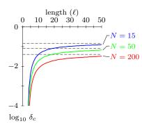
Fig. 3 Asymptotic and non-asymptotic critical accelerations. The critical acceleration  $\delta_c$  (here, in base-10 log scale) is an increasing function of  $\ell$  that approaches its upper bound (dotted line)  $\Delta = \frac{1}{\sqrt{N\pi}}$  when  $\ell = K$ . Here K = 50 and the three curves correspond to N = 15, N = 50, and N = 200 respectively.
