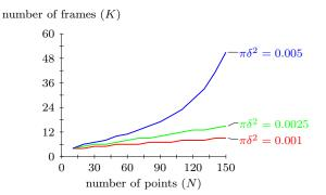
Fig. 5 Minimal number of frames required for detectability. Theses three curves represent, as a function of the number of points N, the minimum number of frames (K) required for a trajectory with length  $\ell = K$  and various values of the maximal acceleration  $\delta$  to be 1-meaningful according to the NFA criterion (15).
